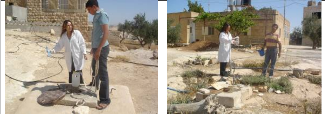
Photos 7& 8: Cistern Water Tests ( Fecal Coliform Test ) Photo Courtesy of ARIJ - 2009
